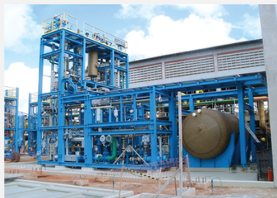
Figure 1. A skid-mounted module forming part of a chloralkali plant. Image courtesy of ThyssenKrupp Uhde Chlorine Engineers. Source: (3)
